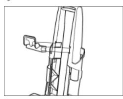
Step 3 Slide the hose caddy into the handle slots and snap into place.
